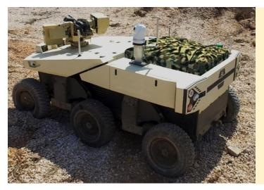
In-hub electric motors Each wheel separately hydraulically suspended Onboard diesel generator battery charger Low silhouette and acoustic signature
